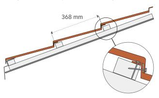
The panels are placed onto battens spacing 368 mm.
